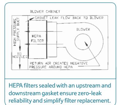
HEPA filters sealed with an upstream and downstream gasket ensure zero-leak reliability and simplify filter replacement.
